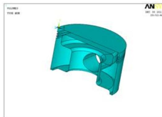
Figure 3.11 Optimized model of piston
