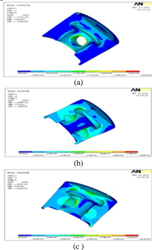
Figure 3.9 Stress at coupled field with 125% load (a) A2168 (b) A4032 (c) Al-GHS1300 alloy pistons
