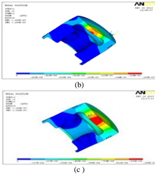
Figure 3.7 Deformation at 250% pressure on (a) A2168 (b) A4032 (c) Al-GHS1300 alloy pistons
