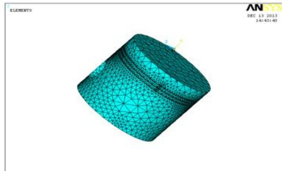
Figure 3.2 Meshing of Piston
